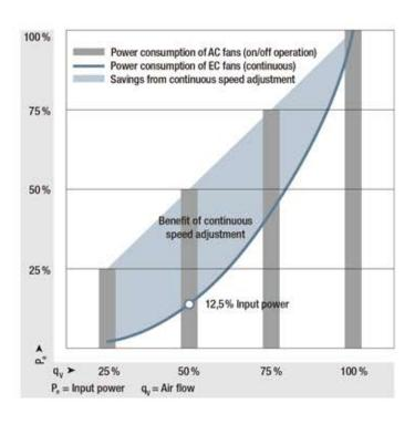
Reduced energy consumption: The bars show the power consumption of fans that are switched on stepwise as needed. Air performance is reduced by 50 % when half of the fans are switched off. The blue line shows the power consumption of all fans with smooth speed adjustment at the required air flow (50 % air flow = only 12.5 % input power).
