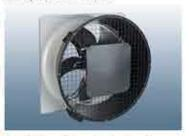
The AxiTop diffuser is designed to recover wasted energy by purposely and efficiently decelerating the flow and reducing swirl, boosting the pressure rise of the impeller. Aerodynamic efficiency is increased and acoustic noise is reduced.
